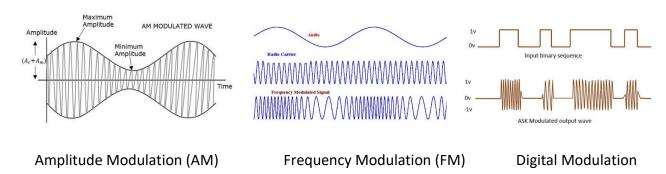
There are many other forms of modulation other than simple amplitude and frequency modulation used in Amateur Radio here are a few:
