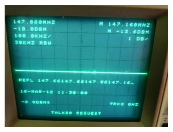
Explanation. This is a spectrum analyzer hooked up to a return loss bridge. This is a picture of the bridge with no load, a reference of -13.6 DBm on 2 meters.
