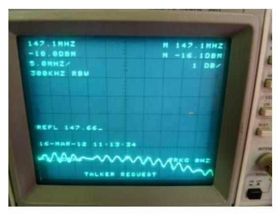
This is a picture of the feedline unterminated. It shows a reading of -16.1 DBm, which is the feed line loss, times two, from -13.6. This comes to 2.5 divided by 2, or 1.25 Db for the line, which is very good.
